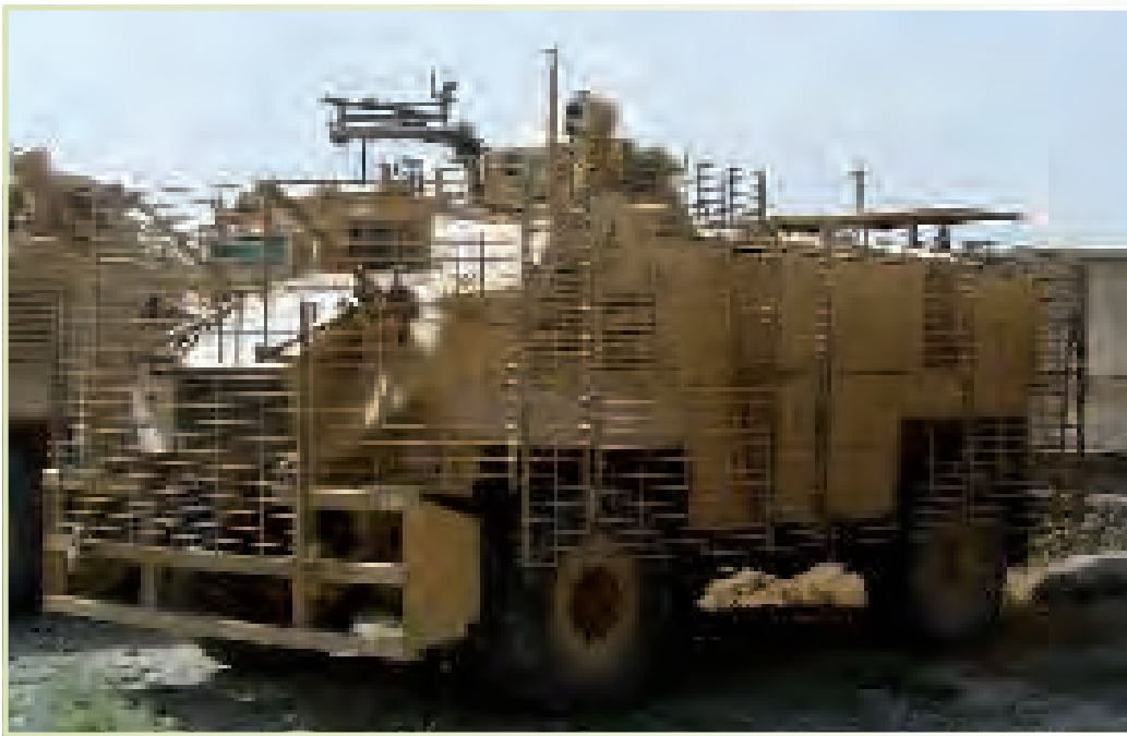
This Saxon was fitted with bar armour.
