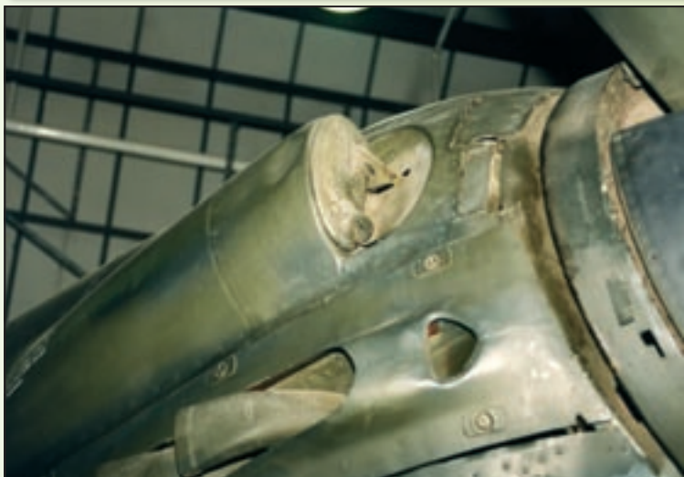
Details of the engine supercharger air intake with tropical filter. Note also details of the exhaust as was used on late D-3 and D-5.
