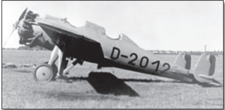
Side view of K48, W.Nr. 3365 with civil registration D-2012. The example shown is powered by a Siemens Sh 20 engine. via R. Michulec.
