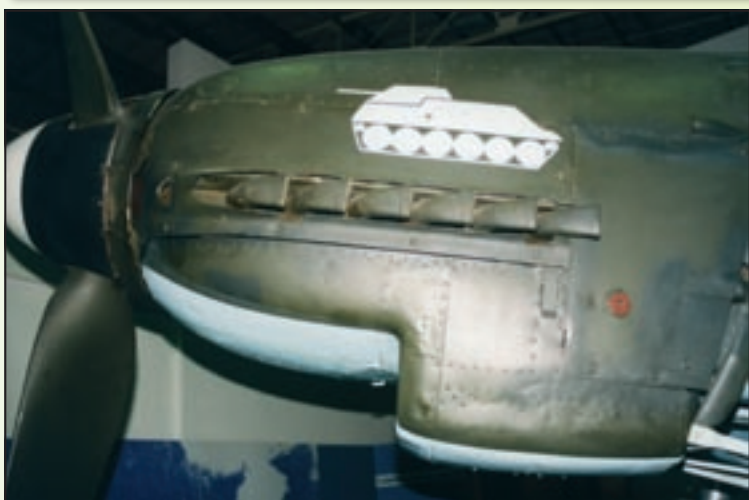
Port side of the engine cowling. Details of the exhaust are visible.
